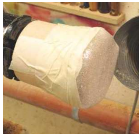
▲ Pic.33 The bowl now needs to be remounted to enable you to remove the marks left by the chuck. A dolly made from a piece of wood covered in bubble wrap and secured with masking tape will act as a friction chuck
